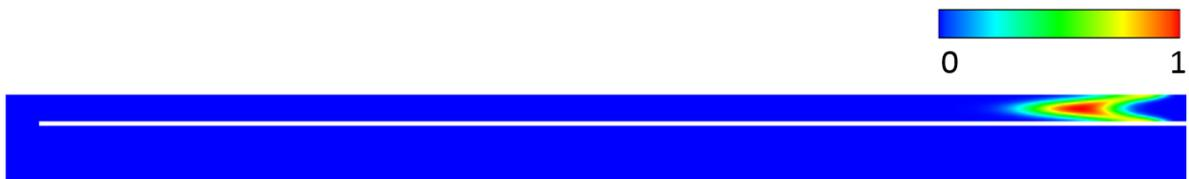
Figure 18: Concentration of tracer injected to outer reactor pipe. Due to symmetrical geometry in axial direction only one half of the entire reactor is modeled.
