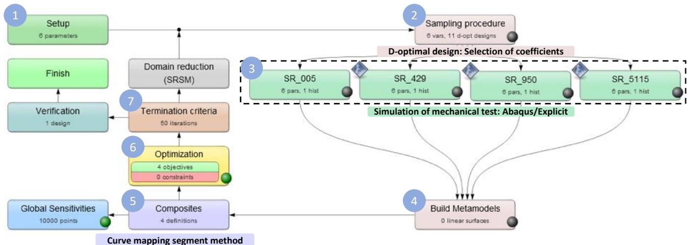
Fig. 4. Optimization-based procedure of the model coefficients determination using the compression tests of cylindrical specimens in Ls-Opt software.
