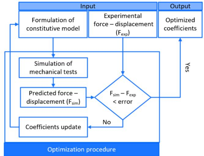
Fig. 3. Flowchart of the optimization-based procedure
