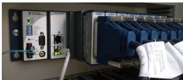
Figure 4: A model of the C-RIO controller with modules.
