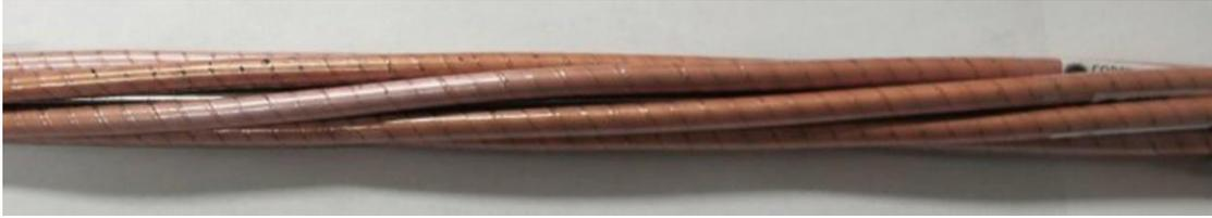
Figure 2.11: Five CORC are twisted together to form a CICC [Corc00].
