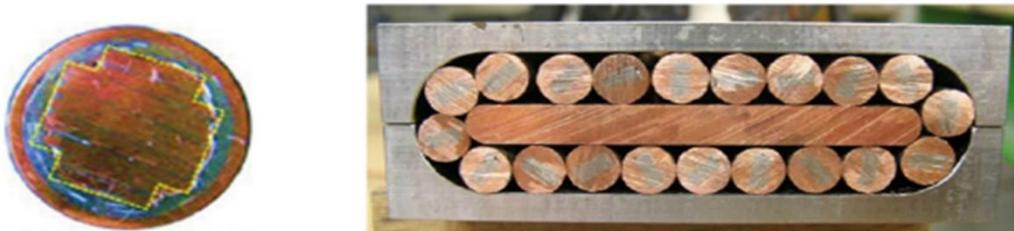
Figure 2.12: Single strand and cabling of TSTC [BFMN18].
