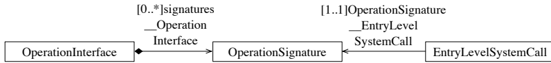
Figure 9.3.: Relationship between an operation interface and the corresponding signatures and entry level system calls - An excerpt from a simplified metamodel based on the PCM [BKR09]
