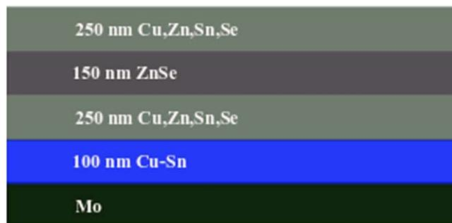
Figure 1. Schematic diagram for a stacked precursor sample.
