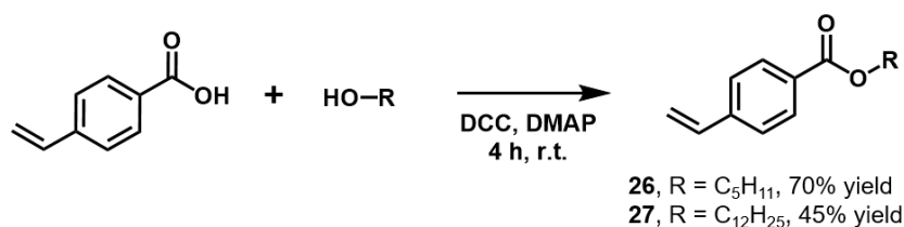
Scheme 3.1. Synthesis route for styrene derivatives 26 and 27 , functionalized with n -pentyl and n -dodecyl residues, respectively.
