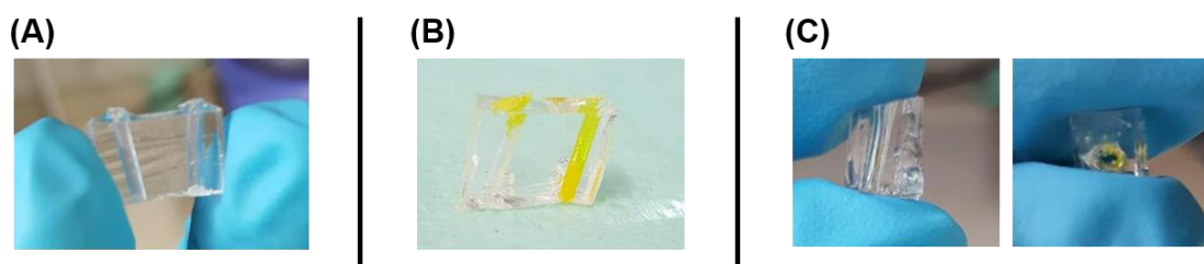
Figure 4.64. (A) Cylindrical PDMS mold used as reactor. (B) Precursor mixture (in DMF) was filled inside the PDMS mold and irradiated 7 h at 320 nm. (C) After washing with solvent, insoluble material was isolated only at the walls of the reactor.
