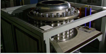
(a) A photo of the GESA cathode and field grading rings in its shielding enclosure.
