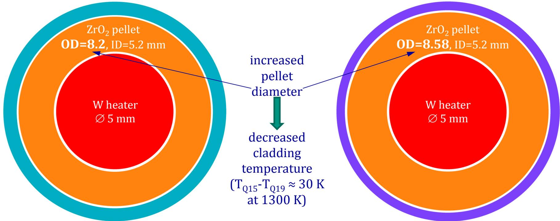
QUENCH-15 (ZIRLO cladding with OD=9.5 mm, Wall Thickness=572  $\mu\text{m}$ )
