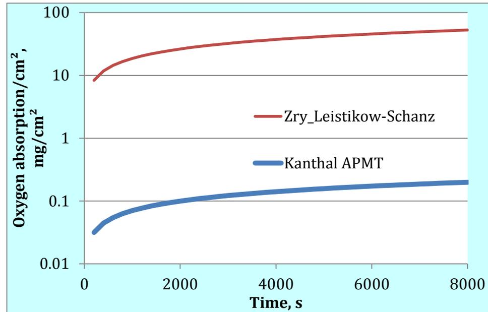
Oxidation in steam at 1200 °C in comparison with Zry-4
