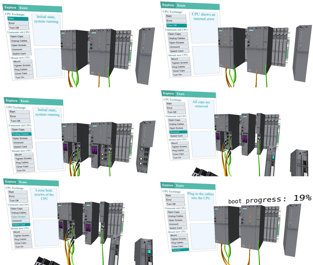
Fig. 6.9: Some of the major steps to exchange the CPU module.
