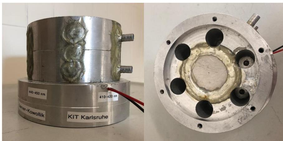
**Figure 70.** Photoreactor used for irradiation with LEDs in the visible light range.
