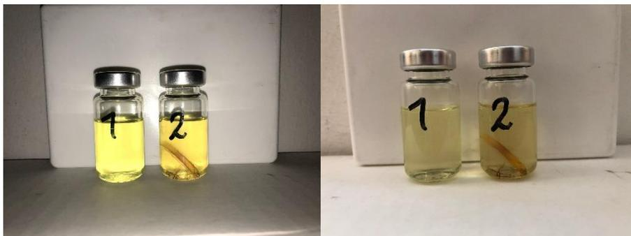
**Figure 161.** (1) Non-irradiated reference. (2) Irradiation styrylpyrene-polymer (P3) film at 410 – 420 nm for 4 h. Subsequent addition of water dissolved the reference 1 while 2 remained solid, successfully proving the cross-linking upon irradiation.
