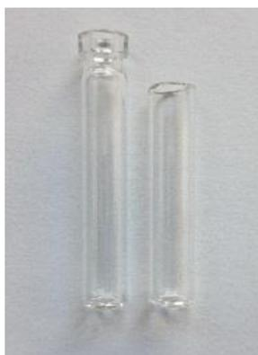
**Figure 73.** Left: uncrimped vial; right: vial after removal of the headspace section.
