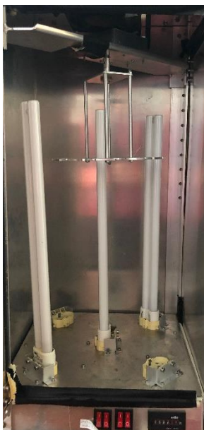
Figure 7.1 – Picture of the employed photoreactor for the hetero-Diels–Alder reaction.
