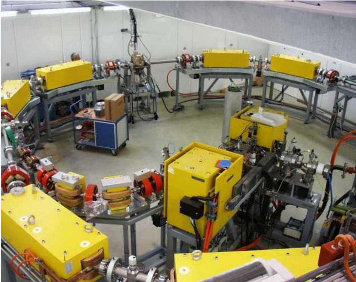
**Figure 3.1.:** Overview of the KARA pre-accelerator chain. The electron-gun is located at the right hand side, from there the electrons are transferred to the racetrack-microtron, its two dipole magnets can be seen in the middle. Afterwards, they are transported through the transfer line to the booster synchrotron that spans along the outer walls.
