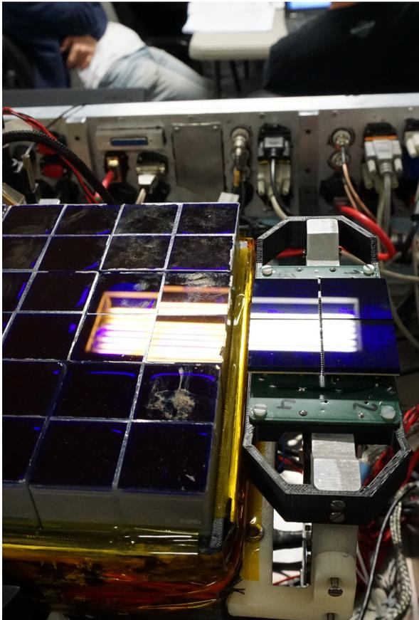
**Figure 5.1:** EUSO-SPB1 PDM and SiECA alignment before cleaning and heater insulation installation
