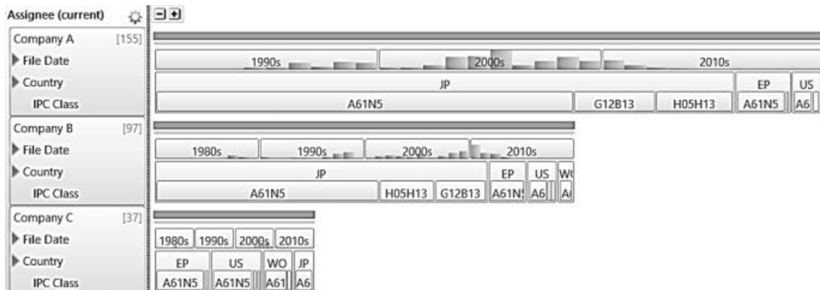
Figure 2.8.: A visualization layout proposed by [112], a so called embedded bar chart. The distribution of metadata attributes in the dataset is represented by a hierarchy of attributes: assignee, then date of filing, then country, then IPC class.
