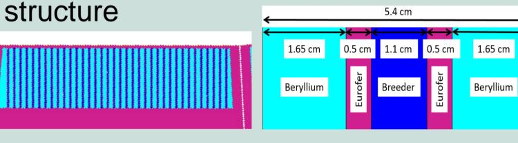
Geant4 Constructive Solid Representation allows replication only within basic shapes  $\rightarrow$  Split into basic shapes; homogenized material for left-over 8.4% of volume
