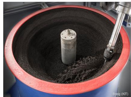
Stream Finishing of a specimen using KXMA 16
