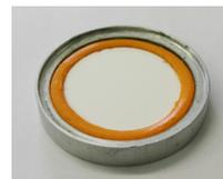
Flexible: 3D printed customized sealing
