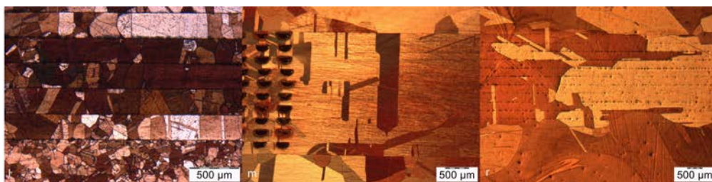
Figure 8. Diffusion bonding of oxygen-free copper, t = 4 h: Left: T = 850 °C. Middle: T = 900 °C. Right: T = 1000 °C.
