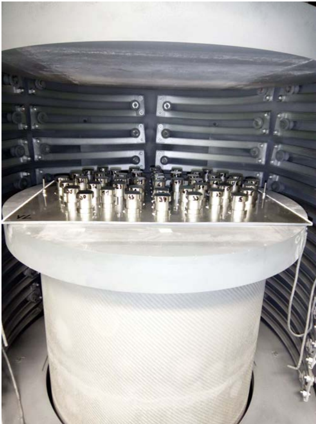
Figure 4. Multi-diffusion bonding of 50 small parts consisting of several dozens of layers in one plane.
