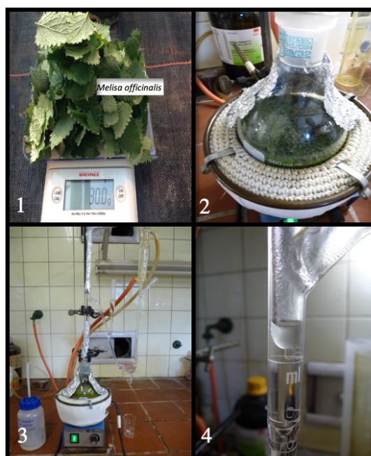
Figure 2.3: Steam Distillation unit for extraction of oil from Mentha plants. The plants were weighed (1), heated in a round bottom flask (2), and the oil was extracted using the distillation unit (3) and finally the oil was collected (4).
