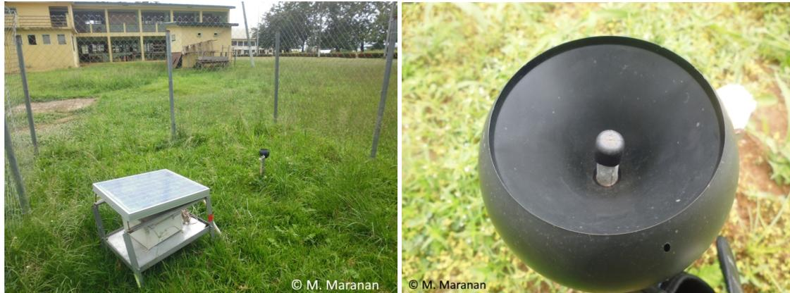
(a) Enclosed rain gauge instrumentation. The solar panel (b) Close-up of a rain collector showing the funnel and a sits on top of a small scaffolding that holds the data logger. thin-wired filter in the middle.
