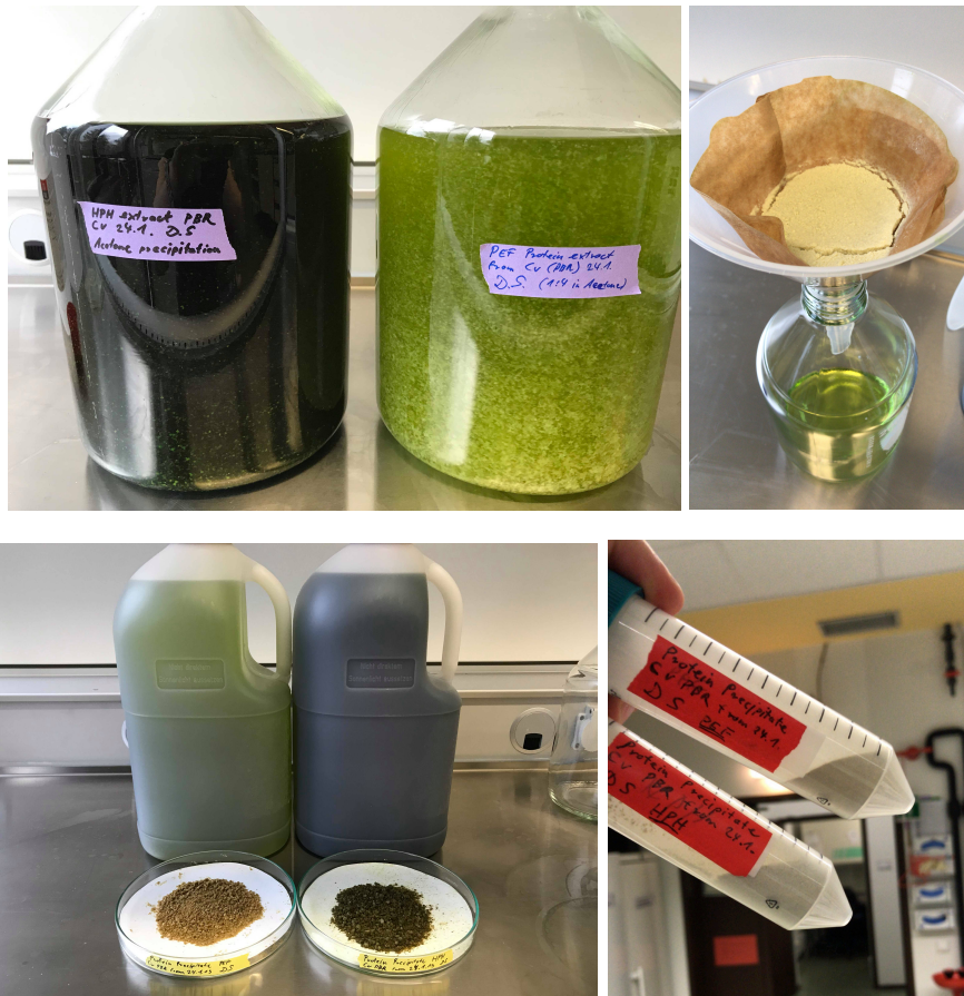
Figure 20: Protein precipitation of extracts obtained by HPH and PEF. The protein fraction obtained from HPH is greener than the fraction obtained via PEF.
