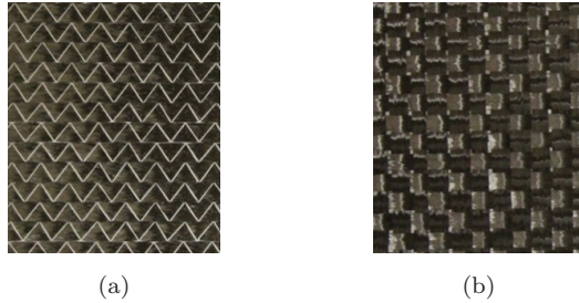
Figure 1.2: Exemplary segment of engineering textiles: Unidirectional (UD) non-crimp fabric (a) and woven fabric (b) [11].
