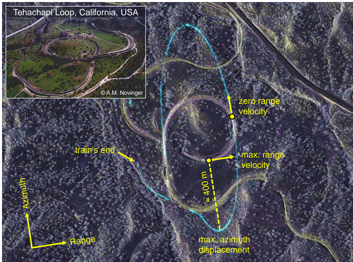
Figure 2.3. Spaceborne SAR image acquired with the TerraSAR-X satellite showing the Tehachapi Loop, in California, USA. A moving train is detected several times with different displacements from its actual positions (especially in azimuth), so that the detections form an ellipse (shown in blue). The azimuth displacements are proportional to the velocity of the train in the range direction.
