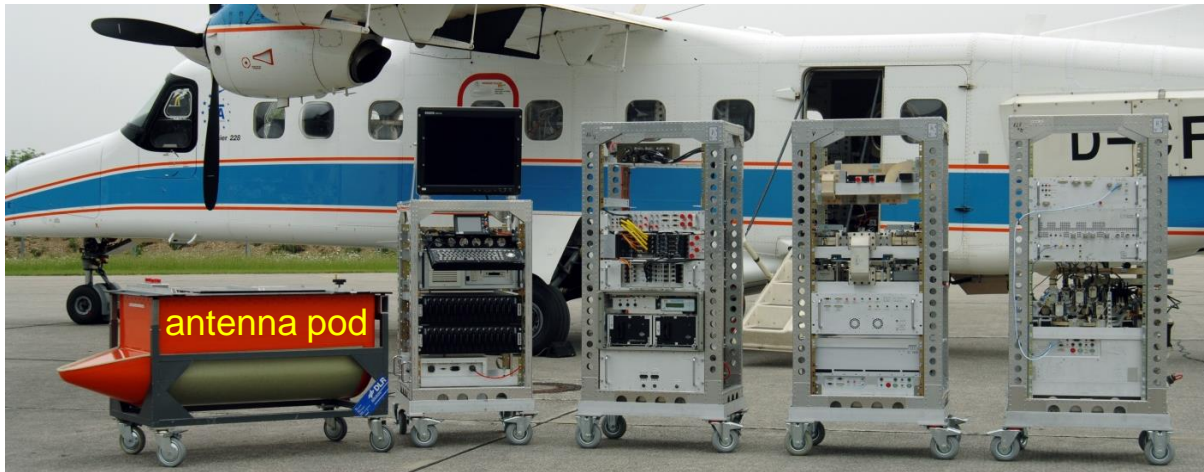
Figure A.3. F-SAR instruments (X-, C-, S-band systems and the antenna pod) before the installation onboard the Dornier DO228-212 aircraft for the first GMTI experiments in February 2007 [146].
