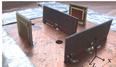
Figure 4.21: Fabricated prototype of the compact MIMO antenna system [22].
