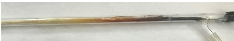
**Fig. 4.4.2:** Conventionally heated fiber with inhomogenous reaction over the length.
