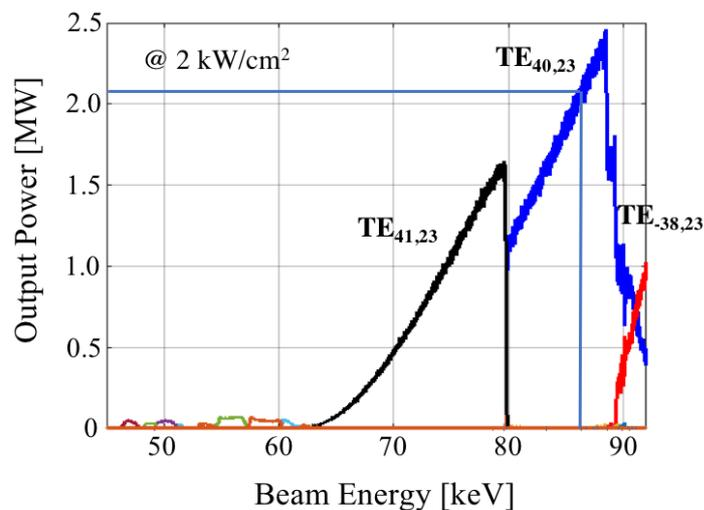
**Fig. 1.3.4.** Start-up scenario at 8.23 T and  $I = 68$  A using the magnetic field distribution of the upcoming 10.5 T magnet and the IMIG at a nominal beam energy of 86.4 keV.
