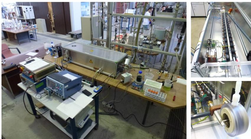
**Fig. 2.1.2:** Pulse Forming Network generator for pilot-scale PEF-processing of microalgae installed at the University of Almería for on-site experiments. Overall view of the installation, left. View into the generator housing onto the 15 element pulse forming network generator in Blumlein configuration, right, upper image. The treatment chamber, mounted at the generators interface consists of a polycarbonate housing and two parallel stainless steel electrodes, right, lower image.
