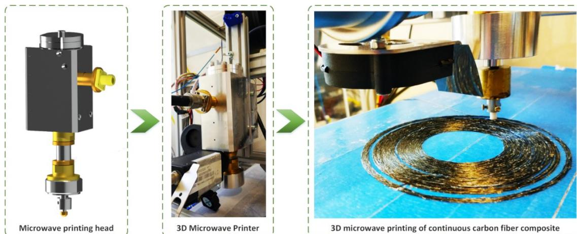
**Fig. 4.7.1:** 3D microwave printing technology of continuous carbon fiber reinforced composites.
