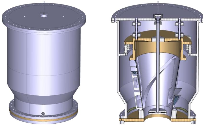
Fig. 1.3.7: Drawings of the preliminary conceptual design of a two-stage ExB MDC.
