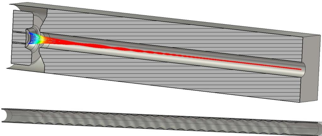
**Fig. 1.7.1:** CUSP-type electron gun with beam tunnel, to be attached to a helical gyro-TWT (top). Cross-section of a helical waveguide structure for a helical gyro-TWT (bottom).
