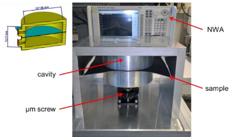
Fig. 4.2.1: Dielectric measurements setup for thin multilayer materials at 2.45 GHz.
