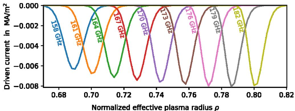
Fig. 1.3.8: Illustration of a first simulation of the localized current drive from the equatorial port of EU DEMO achieved at different frequencies.
