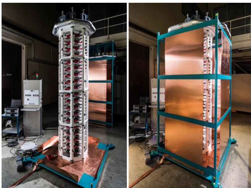
**Fig. 2.2.2:** 9-stage pulse generator for arbitrary waveform generation without current return path (left) and with attached current return path (right).
