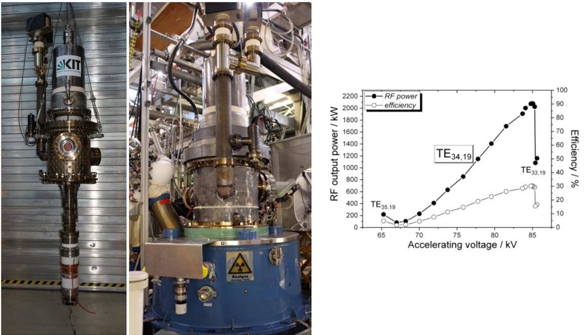
**Fig. 1.3.1:** left: longer-pulse coaxial gyrotron assembly with old diode gun before (left) and after (middle) installation in the superconducting magnet. Right: measured power and efficiency versus the applied accelerating voltage.
