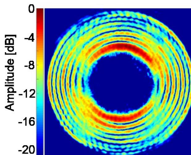
Fig. 1.8.3: Measured amplitude pattern of the TE<sub>28,8</sub> mode operating at 140.006 GHz with a pixel size of 0.2x0.2 mm.
