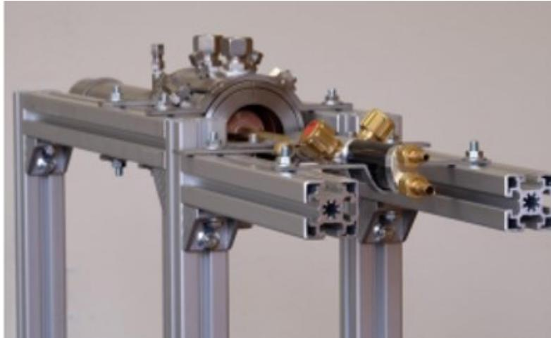
**Fig. 1.3.3:** Test set-up for the performance analysis of the mini-channel cooling concept.
