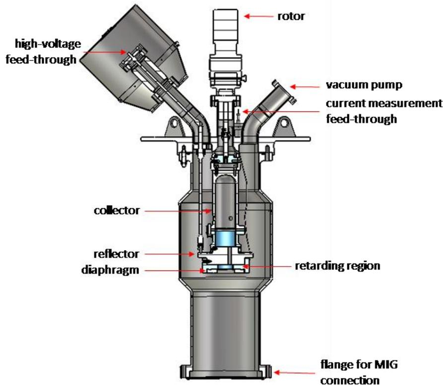
**Fig. 1.8.1:** Representation of the prototype diagnostic device that was manufactured for the study of the beam quality of magnetron injection guns.
