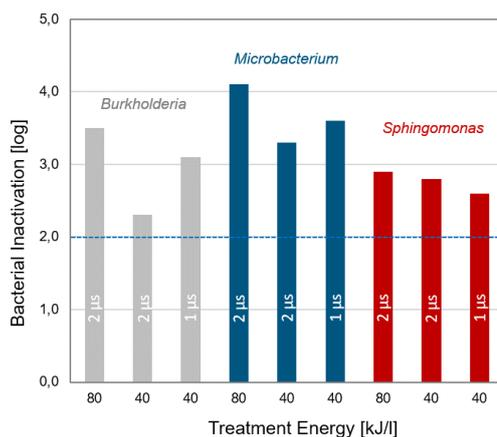
**Fig. 2.1.1:** Inactivation of bacteria isolated from electrocoating lines by PEF-treatment with 1  $\mu\text{s}$  and 2  $\mu\text{s}$  long pulses at a specific treatment energy of 40 kJ/l and 80 kJ/l.
