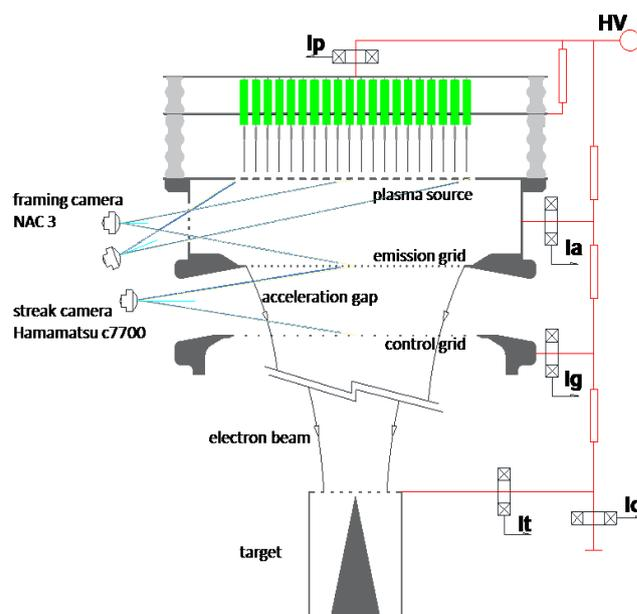
Fig. 2.3.1: Scheme of new cathode combined with high-speed diagnostic equipment
