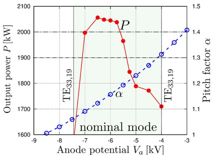
Fig. 1.4.2: Experimental measured output power  $P$  and theoretical pitch factor  $\alpha$  as functions of the modulation anode potential.
