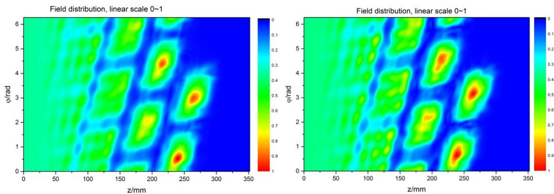
**Fig. 1.3.5:** Field distribution on the launcher wall (linear scale 0~1): operating in the TE<sub>34,19</sub> mode at 170 GHz (left) and in the TE<sub>40,23</sub> mode at 204 GHz (right).
