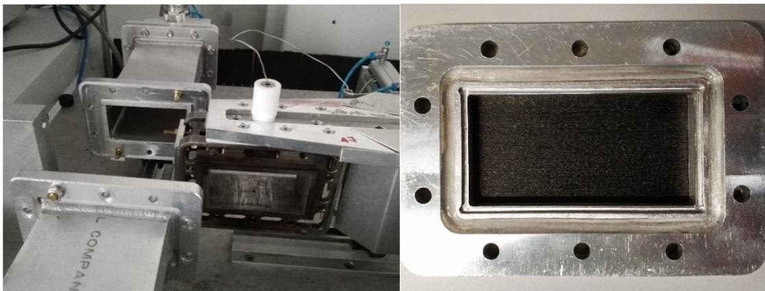
**Fig. 4.6.1:** Left: Transmission reflection test stand; Right: Composite sample in test frame
