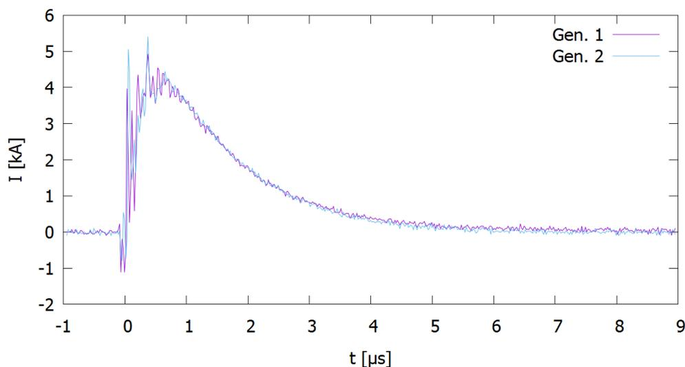
Fig. 2.2.1: Measured pulse currents of both generators.
