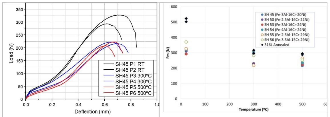
Fig. 3.1.3: Small punch test of AFA alloys showing the ductile behaviour of the new developed material.
