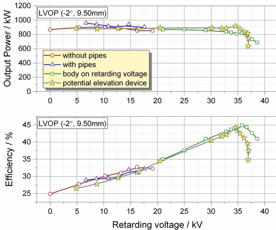
**Fig. 1.2.2:** RF power and total efficiency vs. retarding voltage obtained experimentally with different gyrotron configurations.
