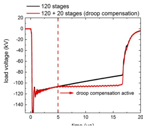
**Fig. 2.2.3:** Output voltage of the generator with droop compensation (red) in comparison to a pulse shape without droop compensation (black).
