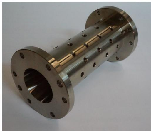
**Fig. 1.2.3:** First prototype of fully metallic beam tunnel
