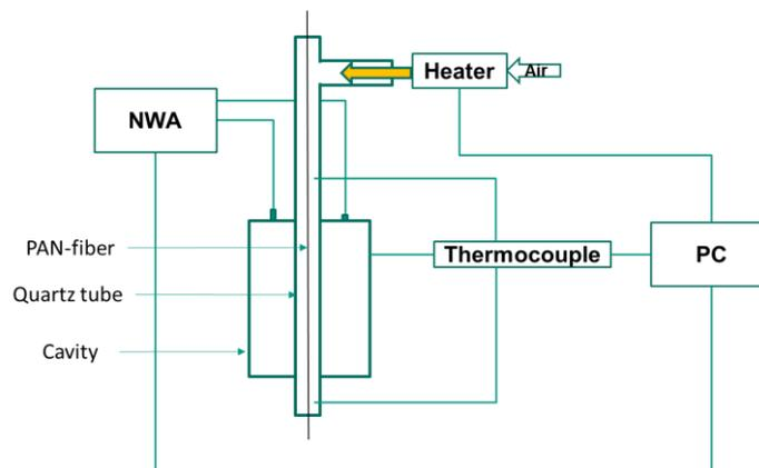
**Fig. 4.4.1:** Schematic of the set up for conventional heating and measurement of the dielectric properties.
