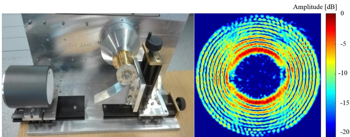
**Fig. 1.1.1:** Mode generator for the TE<sub>28,10</sub> mode (top) and measured normalized pattern (electric field amplitude – vertical polarization) of TE<sub>28,10</sub> at 140.155 GHz (bottom).
