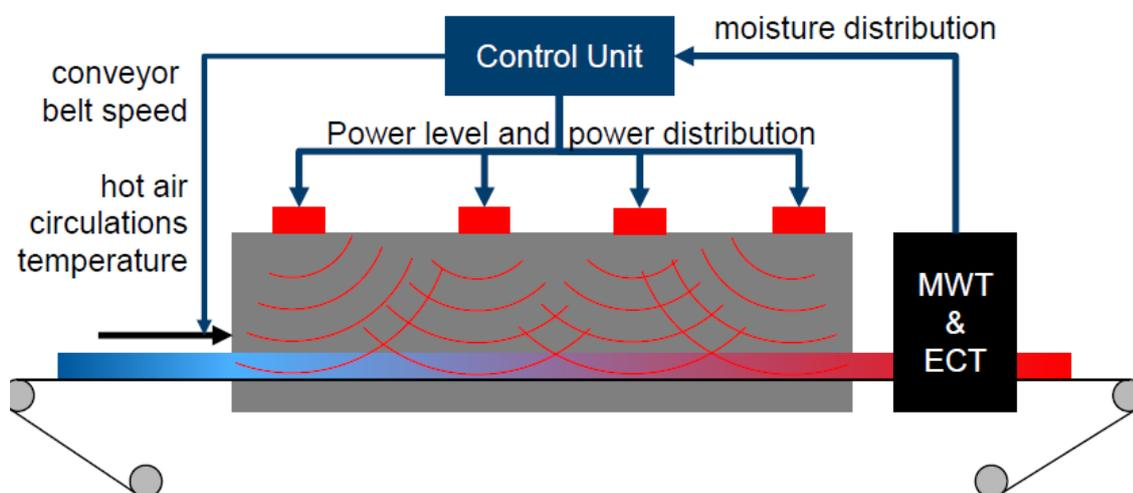
Fig. 4.5.1: Scheme of the microwave drying process and relevant process parameter to be controlled based on MWT or ECT data.
