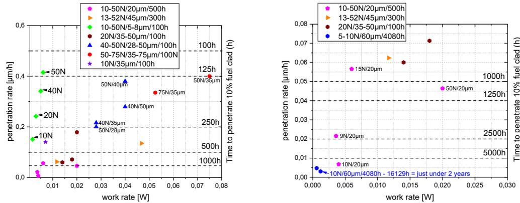
Fig. 3.1.2: Penetration rate vs working rate for different fretting conditions in molten PbBi with 10<sup>-7</sup>wt% oxygen at 400 $^{\circ}$ C; left side without long-term test / right side: with long-term test.
