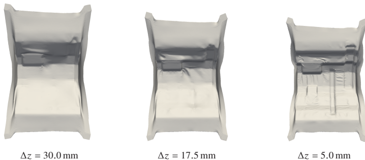
Figure 2.6: Exemplary experimental forming results digitalized by 3D scans for the orthotropic layup and several remaining tool travels \Delta z .
