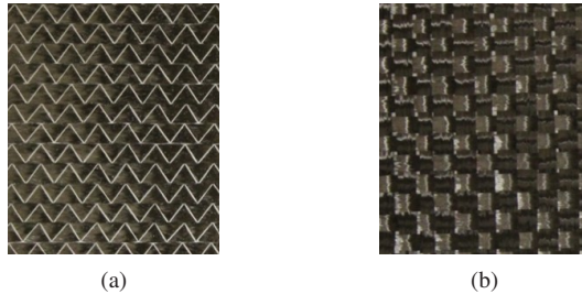
Figure 1.2: Exemplary segment of engineering textiles: Unidirectional (UD) non-crimp fabric (a) and woven fabric (b) [11].
