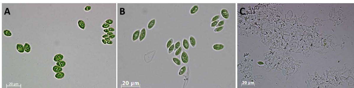
Fig. 7. Microscopic image of microalgae biomass S. almeriensis . (A) Representative images of control untreated S. almeriensis , (B) PEF treated biomass, and (C) HPH treated biomass. Scale bar represents 20 µm.
