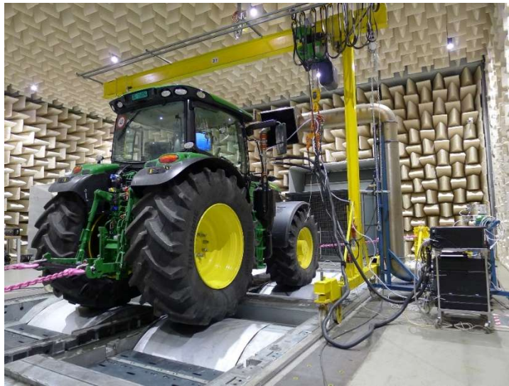
Figure 4: The tractor for field tests is used to reproduce the former fieldwork on the chassis dynamometer
