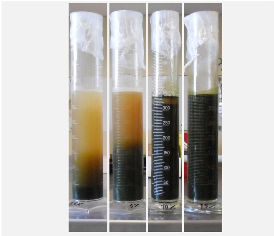
**Figure A3.2 – Particles settling without feed mixing at different concentrations after 100 hours**
