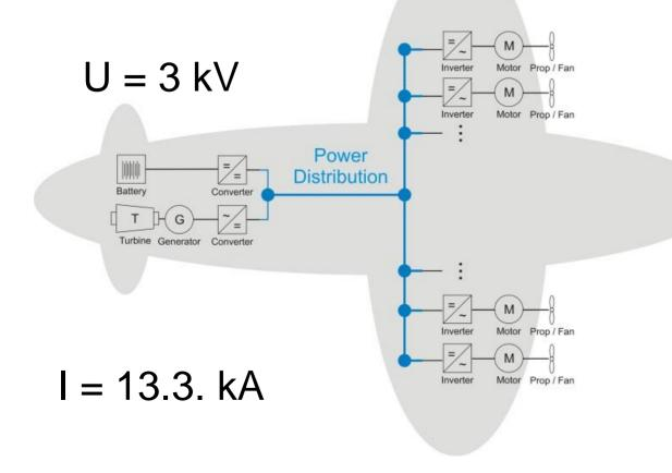
Cable design for 40 MVA DC cable available
