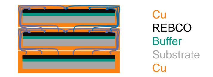
Total contact resistance at T = 77K.  $R = 5.6 n\Omega$  $\rightarrow$  P (13.3. kA) = 0.99 W
