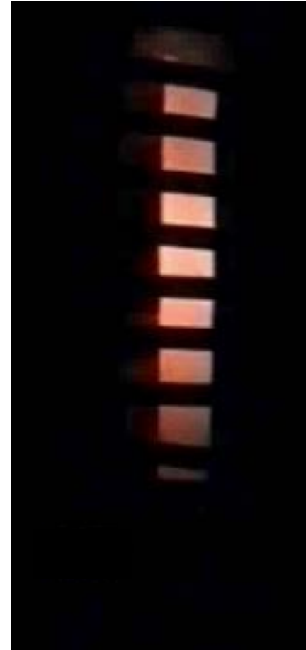
SIC-05 (symmetric rod) Global failure at 1350°C
