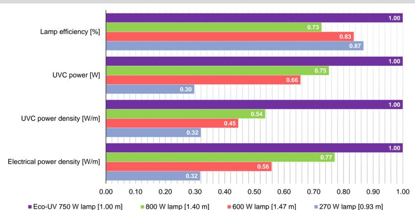
The developed lamp was compared with three commercial lamps in terms of efficiency, UVC output power level, UVC output power density and input electrical power density. The figure shows the normalized values for the comparison.
