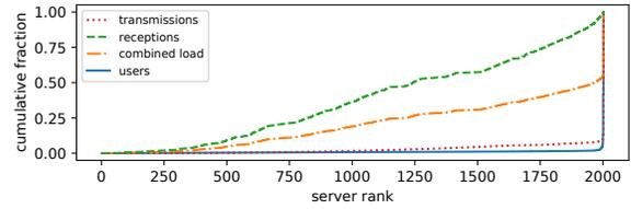
Figure 4. Cumulative fraction of network load per server<sup>6</sup>
