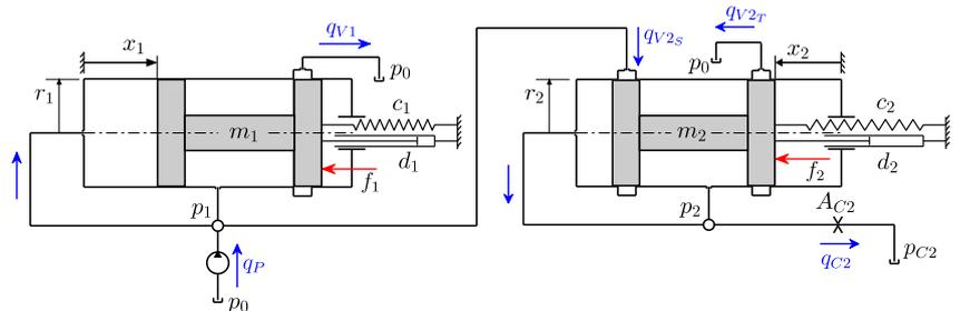
Fig. 2: System under investigation: Two coupled structurally different valves.
