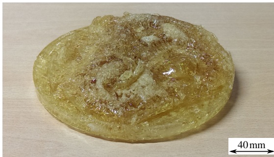
Figure 2.17: Neat UPPH resin after curing trial at atmospheric pressure (Anna Trauth, KIT IAM-WK)
