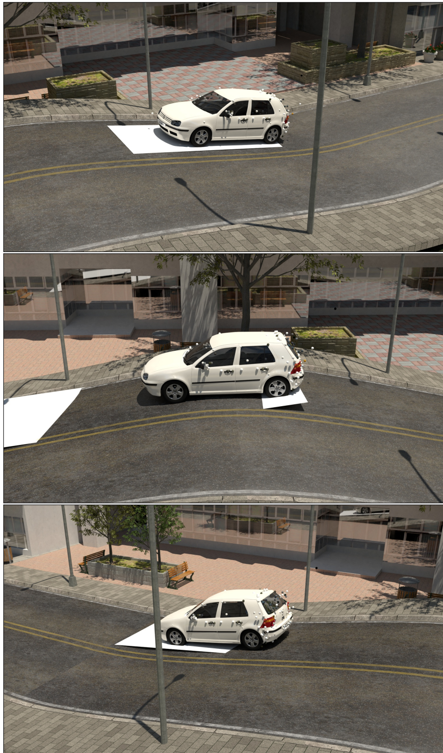
Figure A.3.: Reconstruction results using the trajectory estimation method described in section 6.4.2. The small spheres represent triangulated object points and the white planes the local ground approximations.
