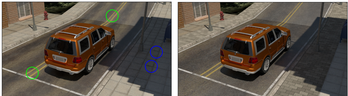
(a) Environment model with repetitive textures. A few examples are emphasized with green and blue. (b) Environment model with procedurally generated textures.
