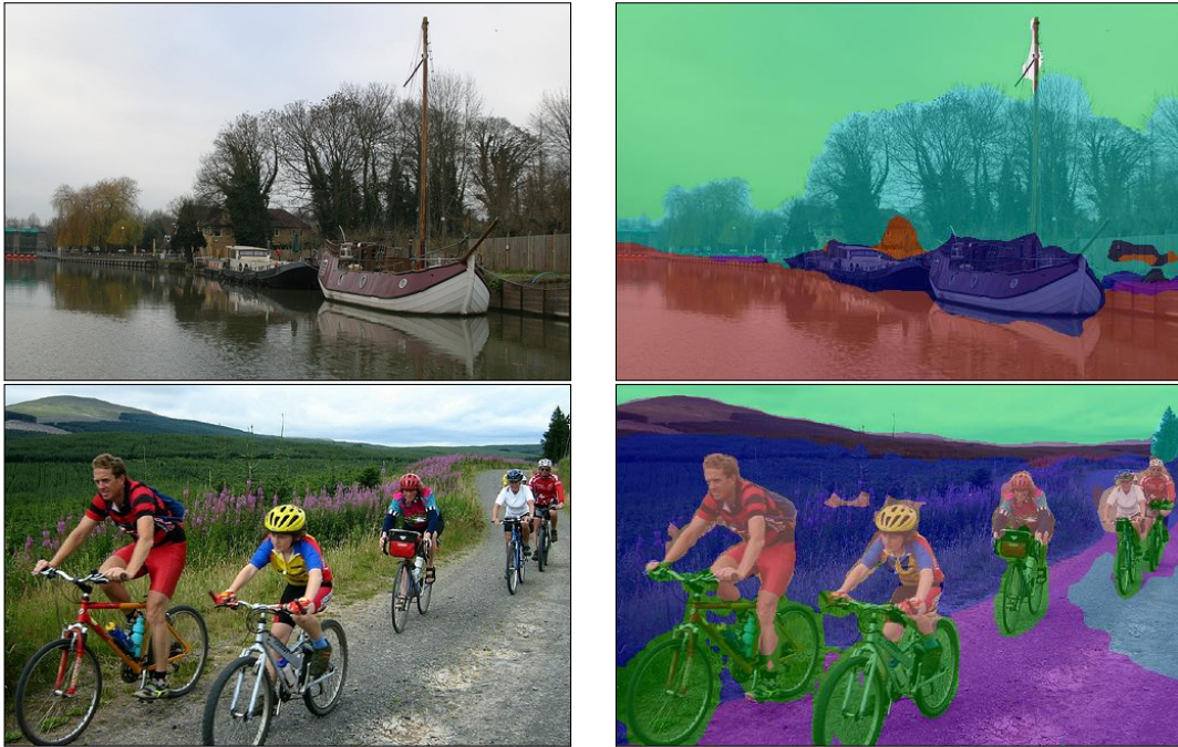
Figure 3.3.: Semantic segmentation examples with images of the Pascal VOC dataset (Everingham et al., 2010) using Long et al. (2015). Each pixel is labeled with a semantic category. The colors highlight different classes. Semantic labels are agnostic to instance information.
