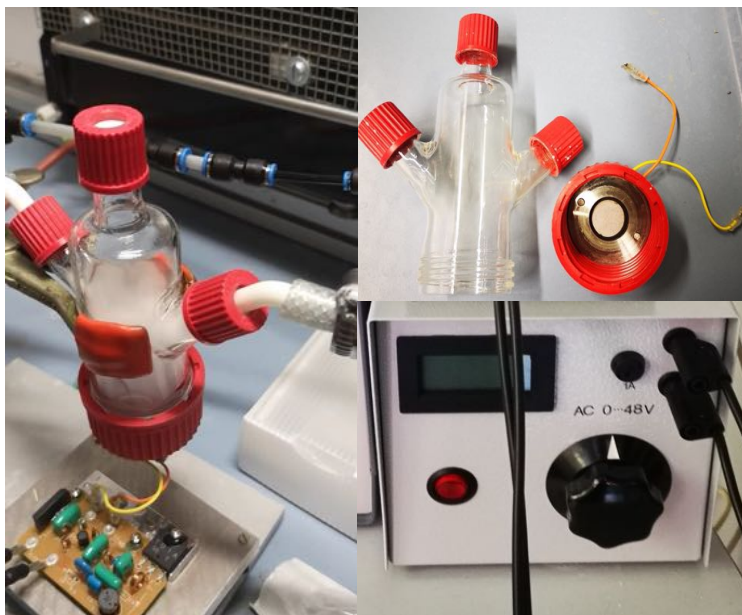
Figure 4.6: Graphdiyne Growth. Photo of the homemade Nebuliser employed for the deposition of the precursors (organic molecules), and the AC power supply adapted to the nebuliser membrane.
