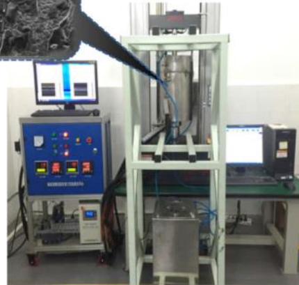
Pebble bed property test apparatus, periodical thermal-mechanical load test
