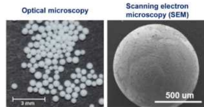
Fig. 1 Former EU reference pebbles, \text{Li}_4\text{SiO}_4 with 2.5 wt.% excess of \text{SiO}_2
