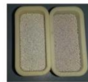
Ceramic breeder pebbles before (left) and after (right) exposure test.
