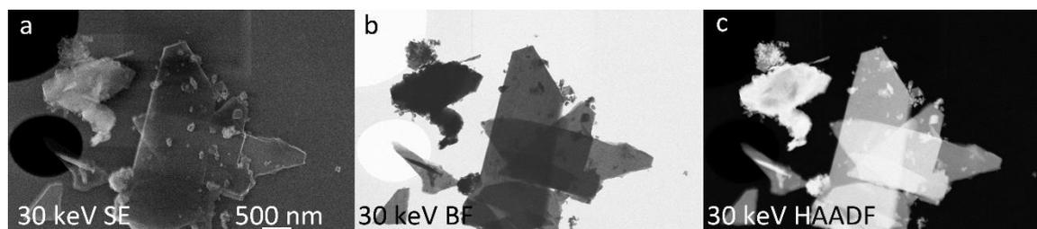
**Figure 4.38.** Low-keV STEM imaging of the same tobermorite region. (a) 30 keV SE-TLD image, (b) 30 keV BF-STEM image, (c) 30 keV HAADF-STEM image. Scale bar in (a) applies to (b,c).
