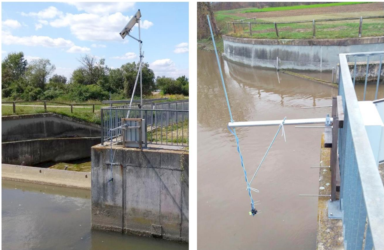
Figure 18: Kraichbach water reflectance monitoring station with a solar panel and a metal switch box containing a car battery and the 'RoX' spectrometer. One downward- and one upward-looking optical cable are installed ~1.5 m above the water surface by means of an aluminum boom.
