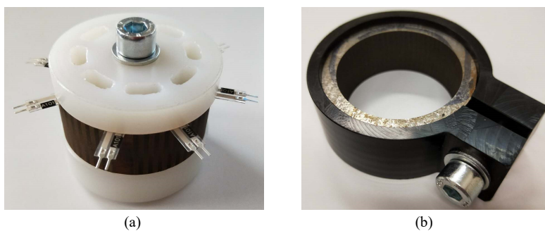
Figure 3.14: Methods to add mechanical stress to the cores. (a) Device to apply axial force. (b) Device to apply radial force.
