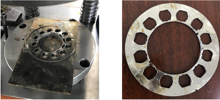
Figure 2.23: Punching results of the non-annealed amorphous stacks.
