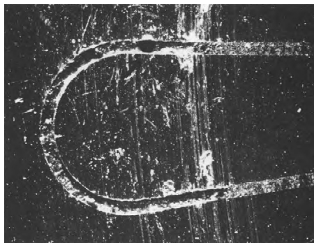
Figure 2.15: Typical deterioration of the glass insert after casting [105].
