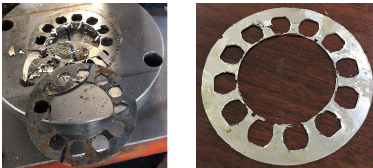
Figure 2.22: Punching results of the annealed amorphous stacks.
