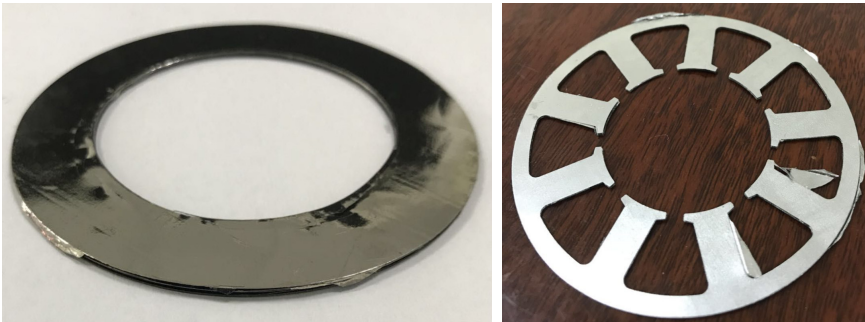
Figure 2.24: Punching results of the non-annealed amorphous stacks with different punching dies.
