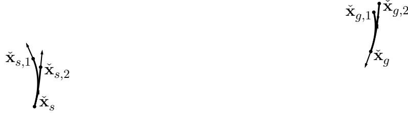
Figure 2.23 Propagation of the start state \check{\mathbf{x}}_s and the goal state \check{\mathbf{x}}_g to the intermediate states \check{\mathbf{x}}_{s,i=1:2} and \check{\mathbf{x}}_{g,j=1:2} with zero and maximum curvature.
