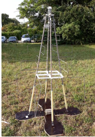
**Figure 5.9:** SKALA version-2 antenna in the South Pole design deployed in the hybrid engineering array at KIT without middle pole and snow spikes.
