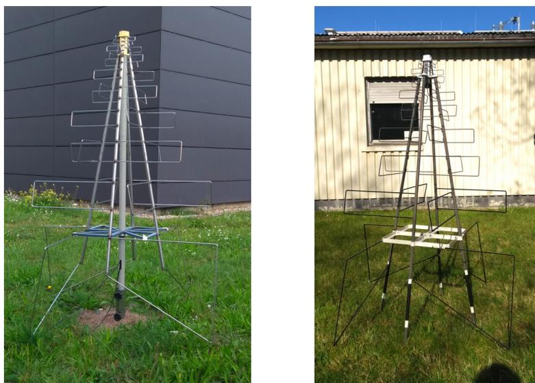
**Figure 5.1:** Left: SKALA version-1 antenna deployed at KIT. Right: SKALA version-2 antenna deployed at KIT
