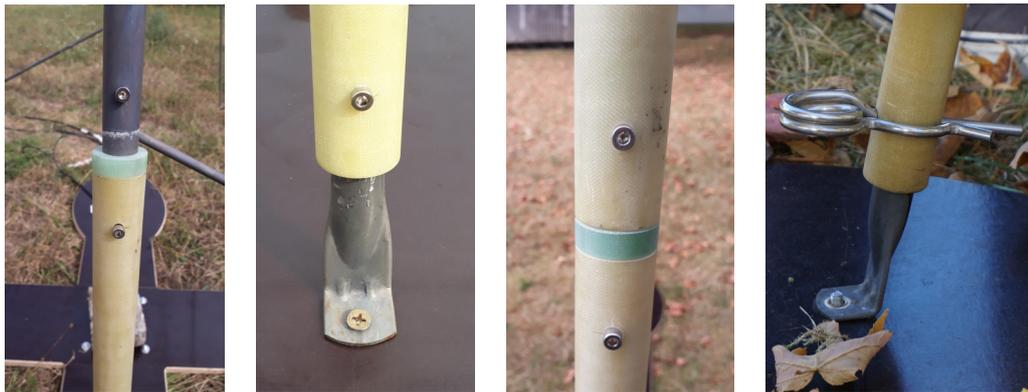
**Figure 5.10:** Details of the SKALA version-2 South Pole mechanical structure. **Left:** Connection between antenna arm and GFK leg. **Middle left:** Connection between GFK leg and antenna foot. **Middle right:** Connection between two GFK legs using a GFK adapter. **Right:** Final connection of a GFK leg to the antenna foot using a cottor pin.
