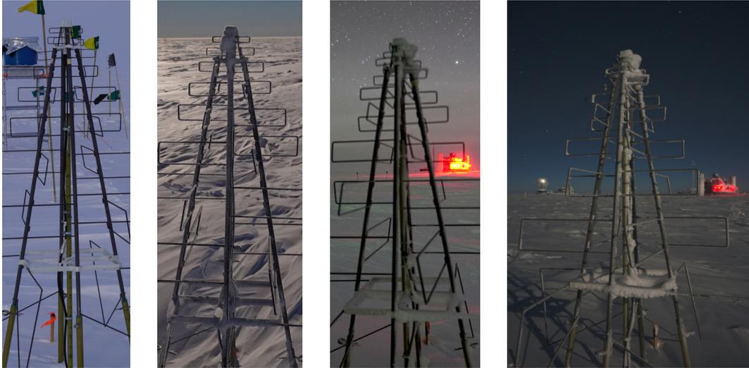
**Figure 8.6:** Snow accumulation on the antenna structure of the small antenna in March, April, May and June 2019 (from left to right) [110].
