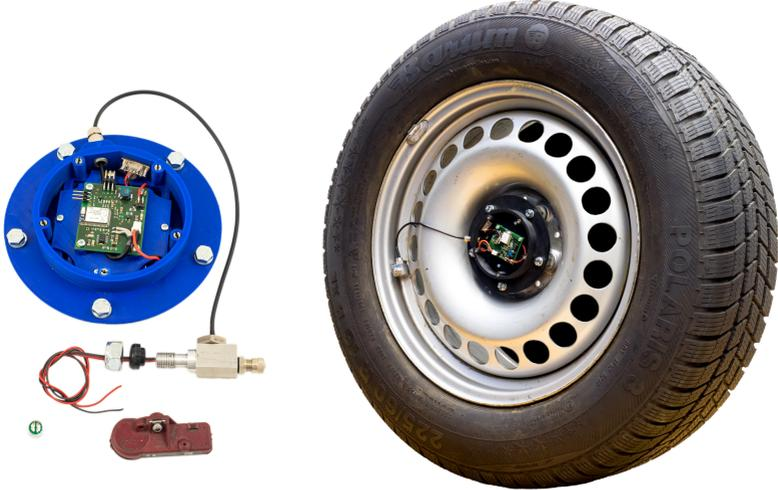
(a) telemetry system without wheel                      (b) telemetry system attached to the wheel
