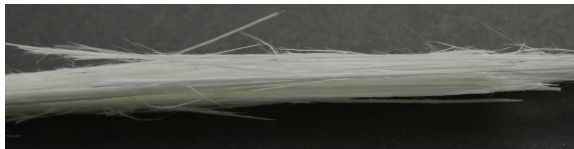
Figure 3.18: Side view of a UD specimen failed under longitudinal tension.
