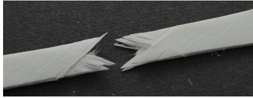
Figure 3.27: Failed \pm 45^\circ off-axis specimen after tensile test. Close-up view of fracture area.
