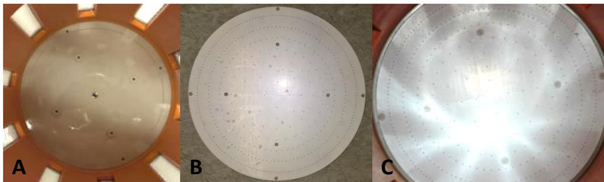
**Figure 57: Bottom plate and gas sparger of pilot scale reactor**
