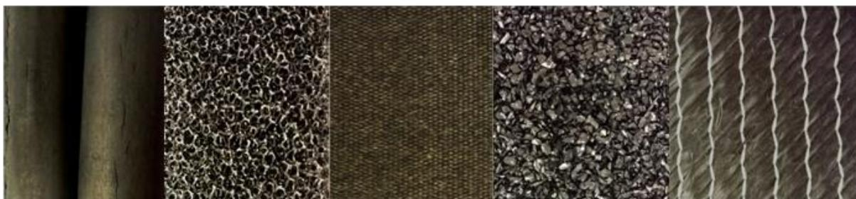
**Figure 53: Different electrode materials**
