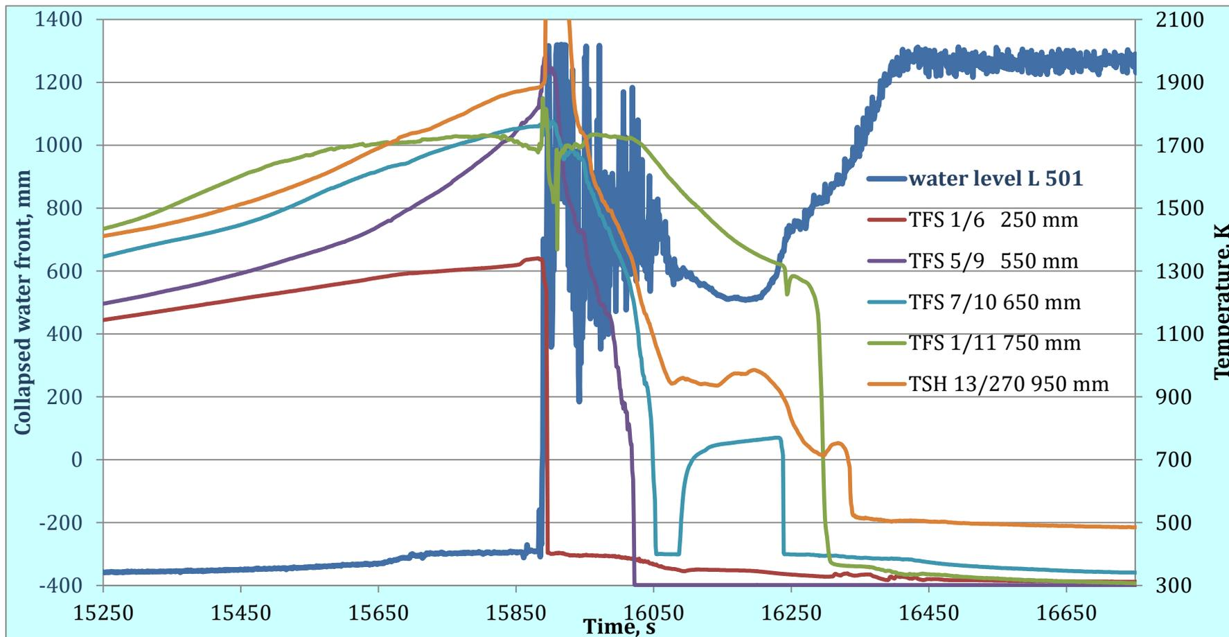
**delayed cooling of the bundle (>450 s) due to filling of insulation annulus through the shroud breach at  $\approx 550$  mm**
