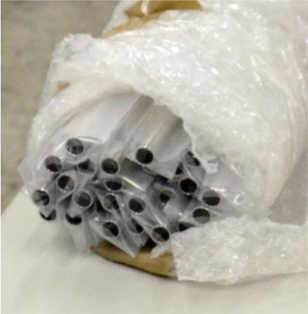
claddings (Zry-2 with inner ZrSn liner)
