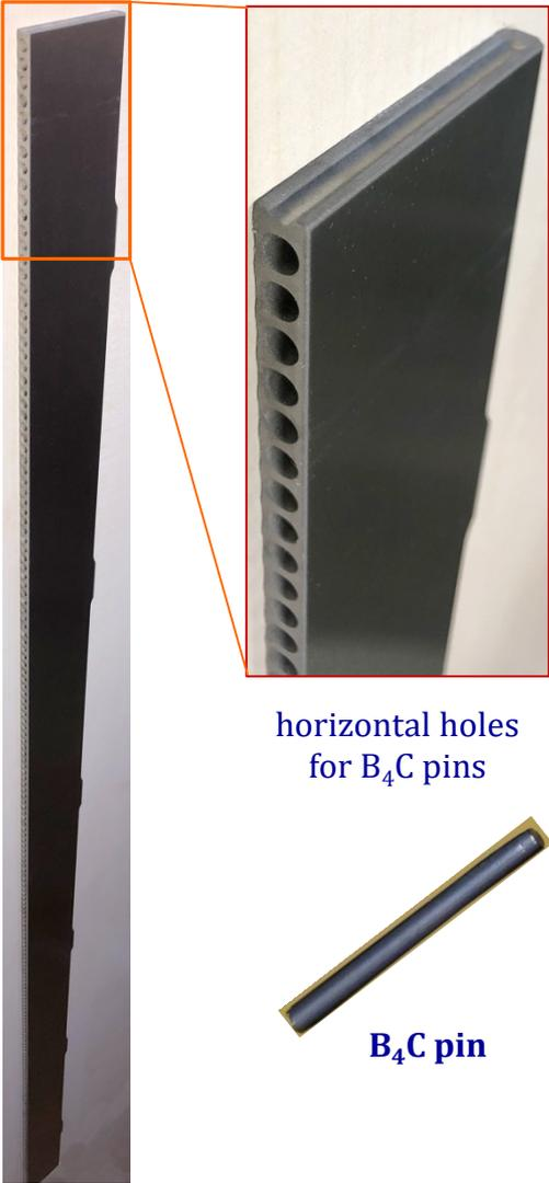
horizontal holes for B<sub>4</sub>C pins
