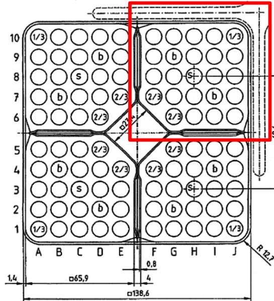
*SSM proposal: study of high temperature degradation of BWR assembly mock-up in QUENCH facility (melt formation due to eutectic material interaction inside absorber cross)*
