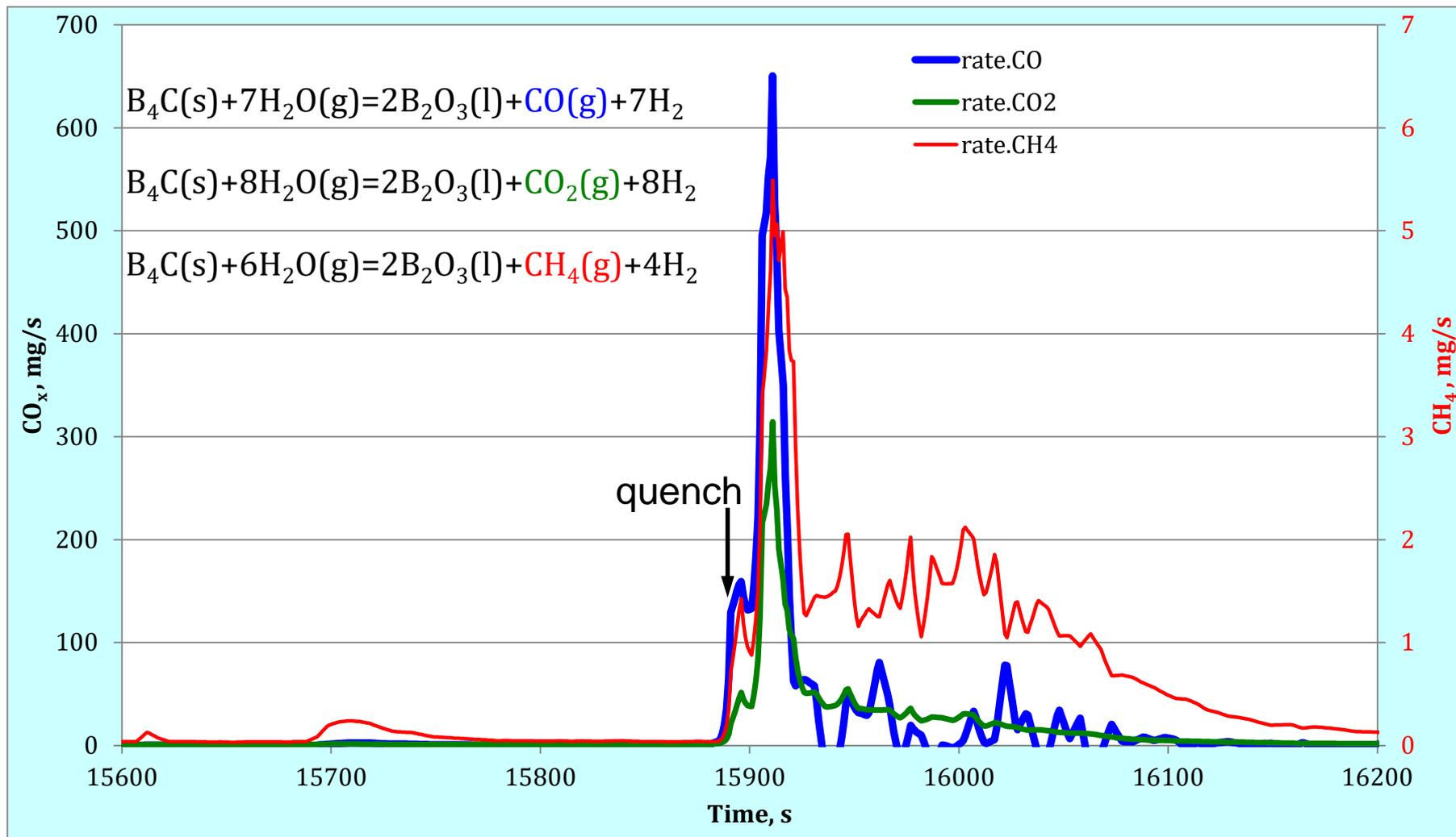
only small release of CH<sub>4</sub> before quench;
