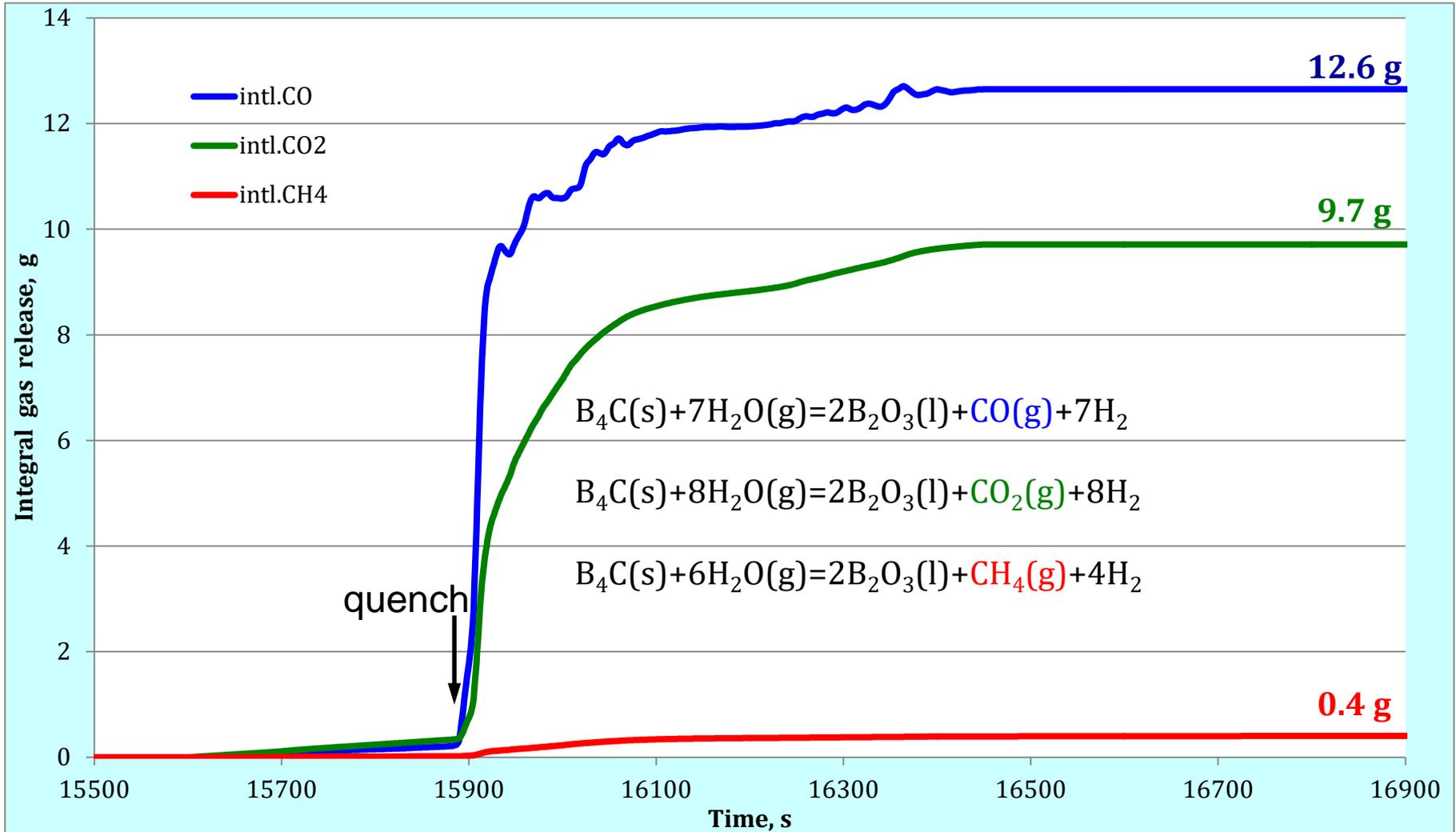
According to CO<sub>x</sub> and CH<sub>4</sub> release: corresponding mass of B<sub>2</sub>O<sub>3</sub> is 96.8 g; H<sub>2</sub> is 10.0 g
