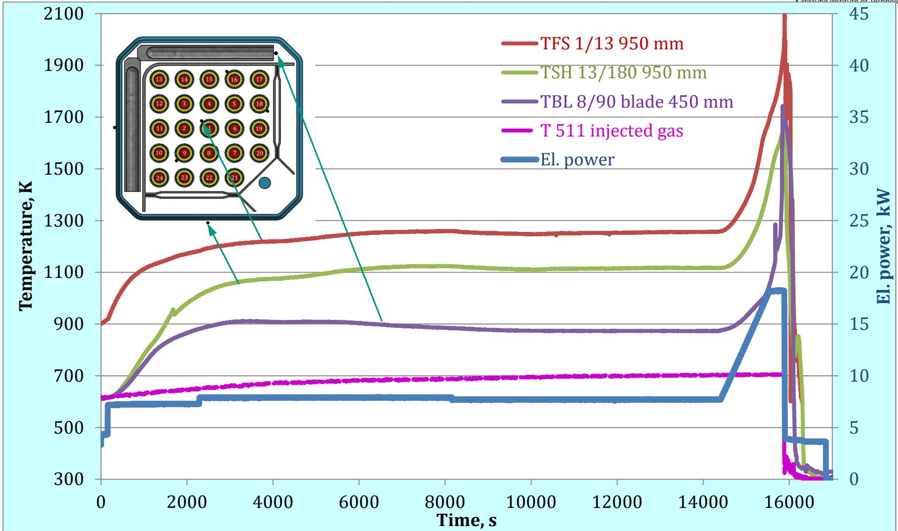
**gas injection: Ar 3g/s during the whole test; superheated steam 3 g/s until the quench initiation**
