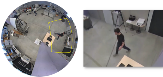
Fig. 2. View synthesis from panoramic color images. A virtual rectilinear camera image (right) is created from a highly distorted spherical image region (left).
