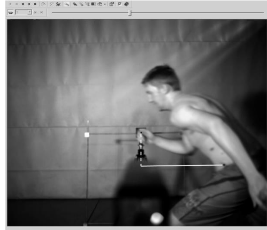
Figure 5.3 The athlete's right hand breaks the beam (marked by the flashing of the timing light at the bottom of the picture) before the hip does.
